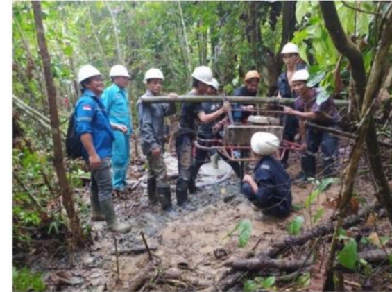
Shot hole drilling
