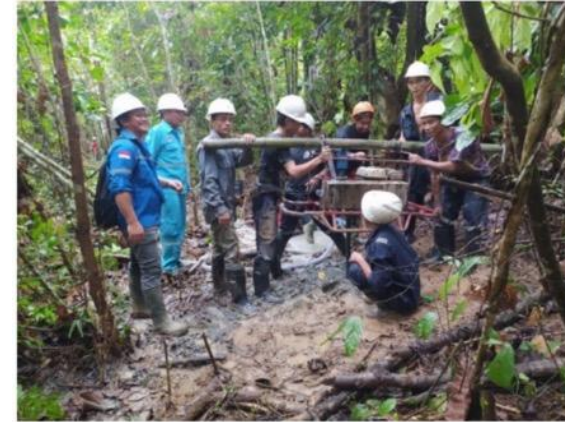
Shot hole drilling
